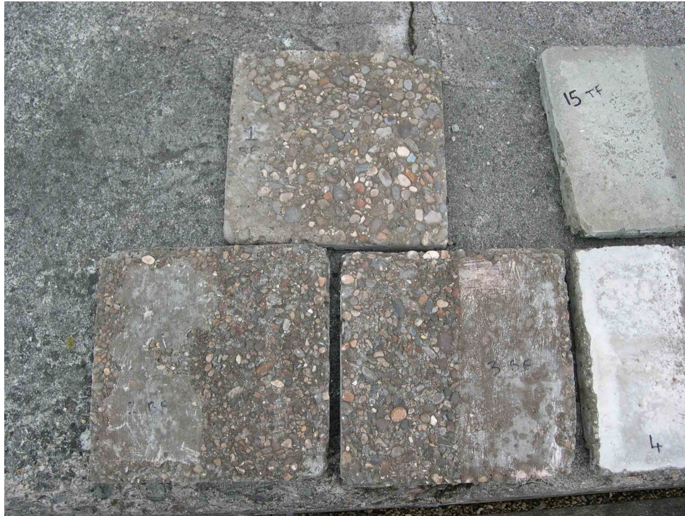
Figure C-1 Flag library using different constituents for the test concrete. Some of the flags used retardants together with post-brushing of the surfaces.
