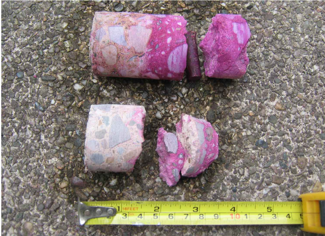
Figure A-21: Carbonation testing of two cores taken from the Bear Ravine.
