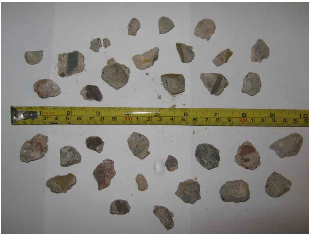
Figure 10: An example of the different types of aggregate used in the concrete mix.
